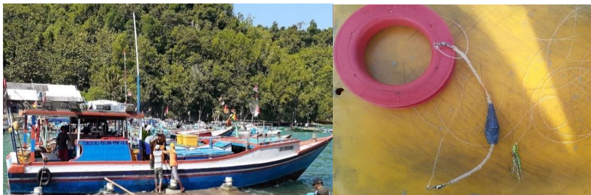
Figure 9. Fishing boat equipped with handline (Original photos).
