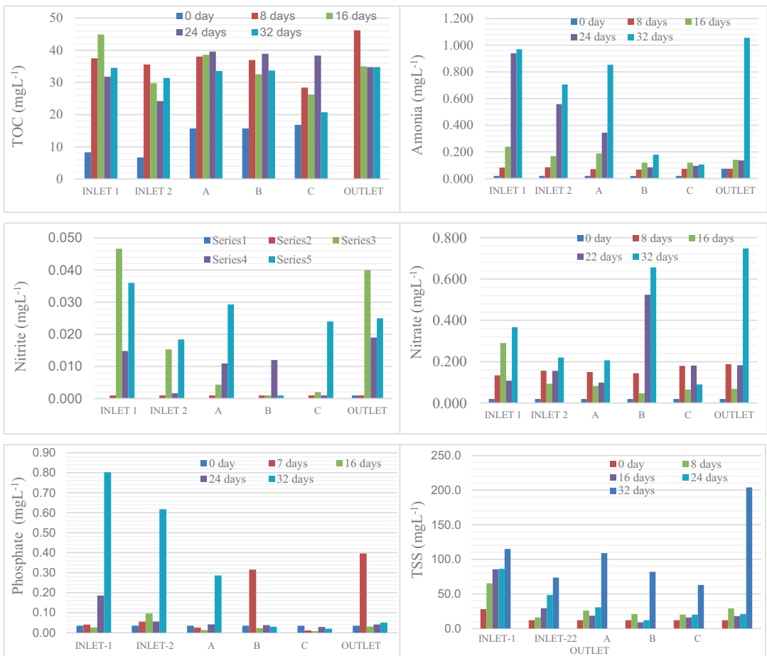
FIGURE 2 Observation of water quality in tiger shrimp aquaculture with different stocking densities and cultivation systems Simple recirculation. (A. 2000 \text{ ind./m}^3 ; B. 1500 \text{ ind./m}^3 , and C. 1000 \text{ ind./m}^3 ).
